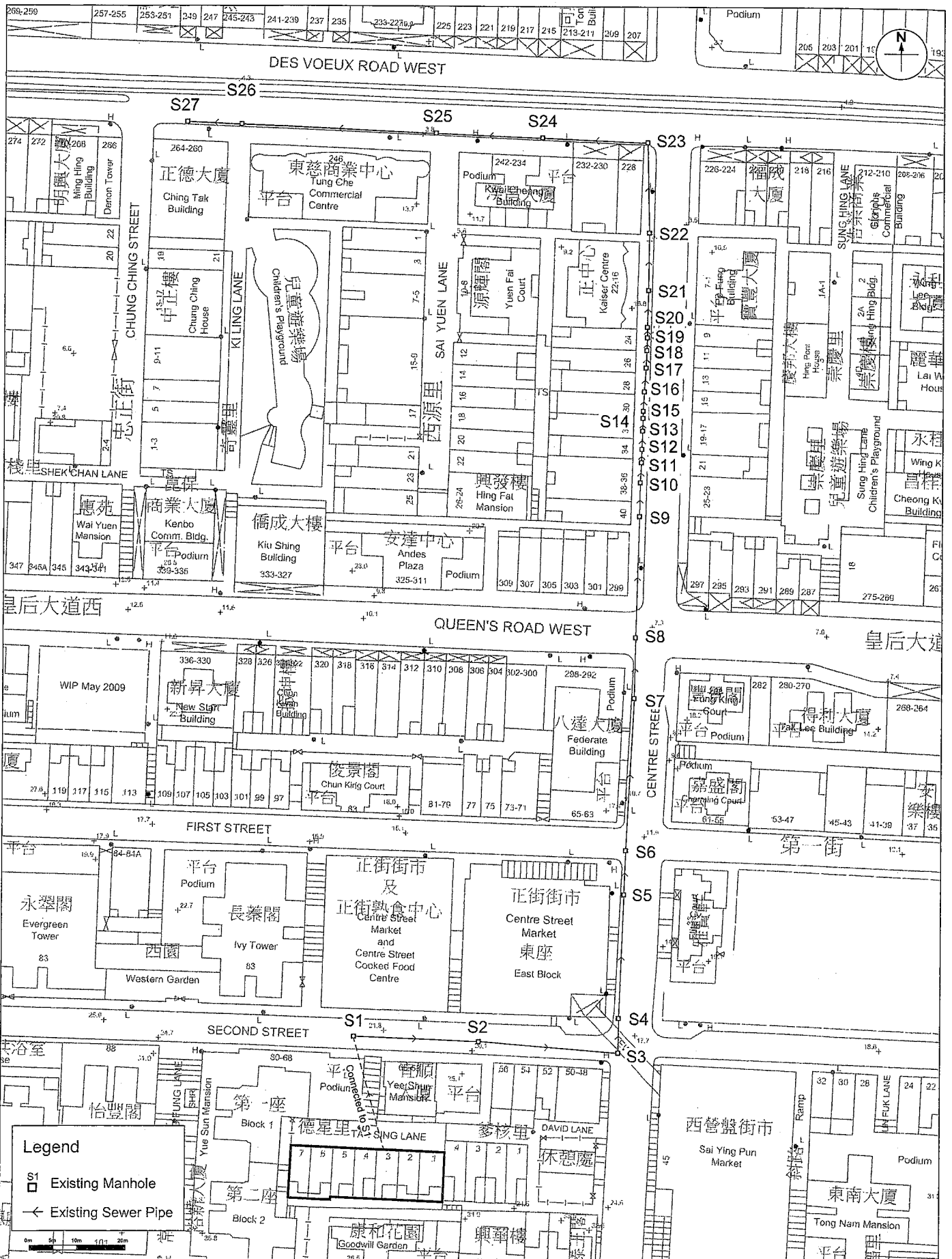
Figure: 2 Title: Existing Sewerage System in the Vicinity of the Subject Site Project: Sewerage Impact Assessment for the Proposed Residential Development at No. 1-7 Tak Sing Lane, Sai Yin Pun, Hong Kong
