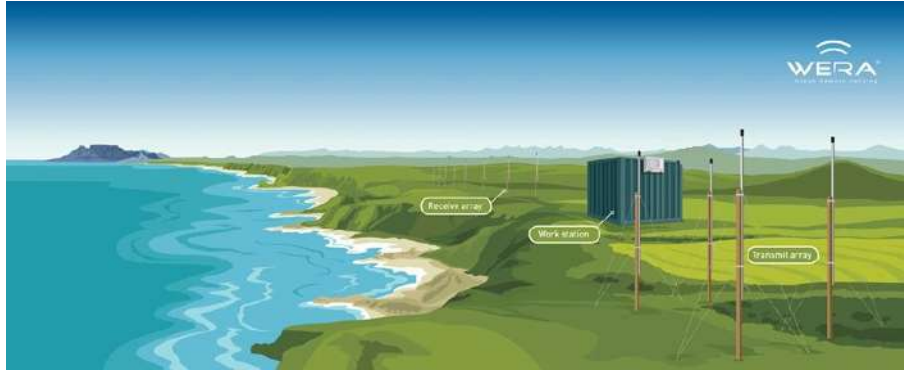
Figure 2: Sketch of WERA Ocean Remote Sensing System.
