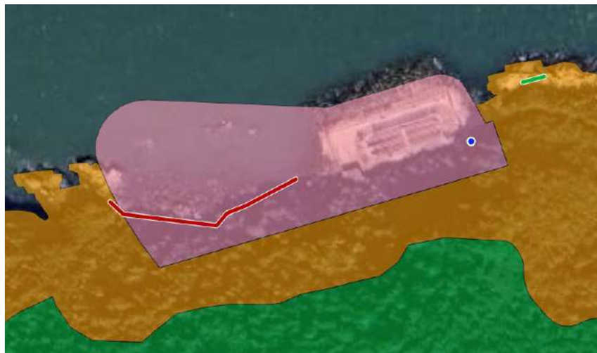
Figure 11: Outline Zoning Plan. Pink: Other Specified Uses; Orange: Coastal Protection Area; Green: green belt. The red and green line represents the Rx and Tx positions, respectively. The power connection is marked by the blue dot.
