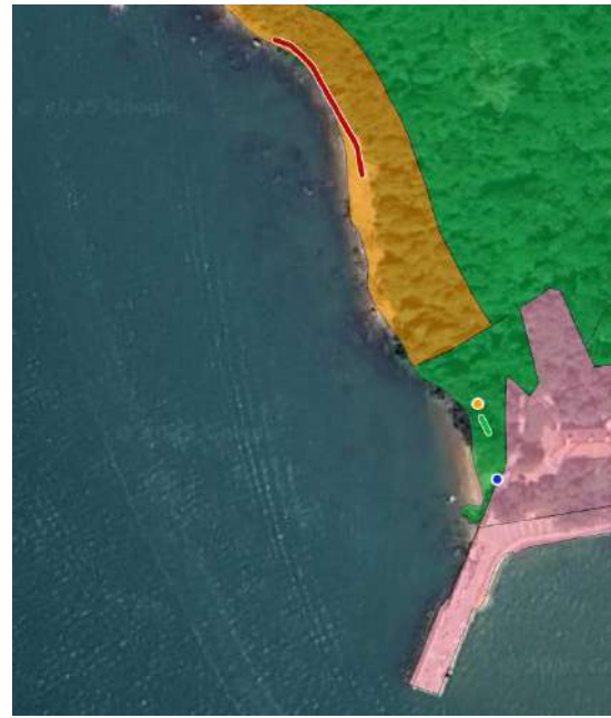
Figure 20: Outline Zoning Plan. Pink: Other Specified Uses; Orange: Coastal Protection Area; Green: green belt. The red and green line represents the Rx and Tx positions, respectively. The server room is marked by the orange dot, whereas the blue one indicates the power connection.
