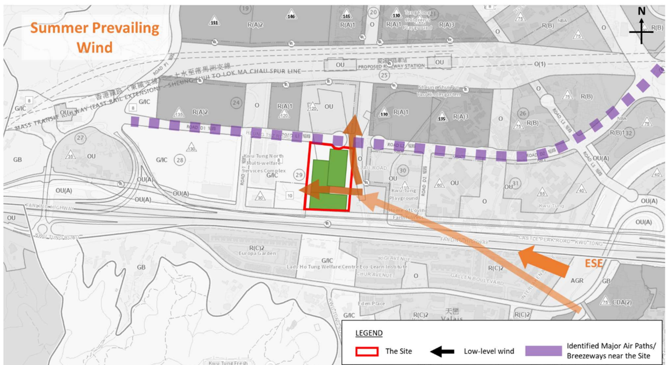
Figure 18 Major Air Paths under Proposed Scheme (ESE Wind)
