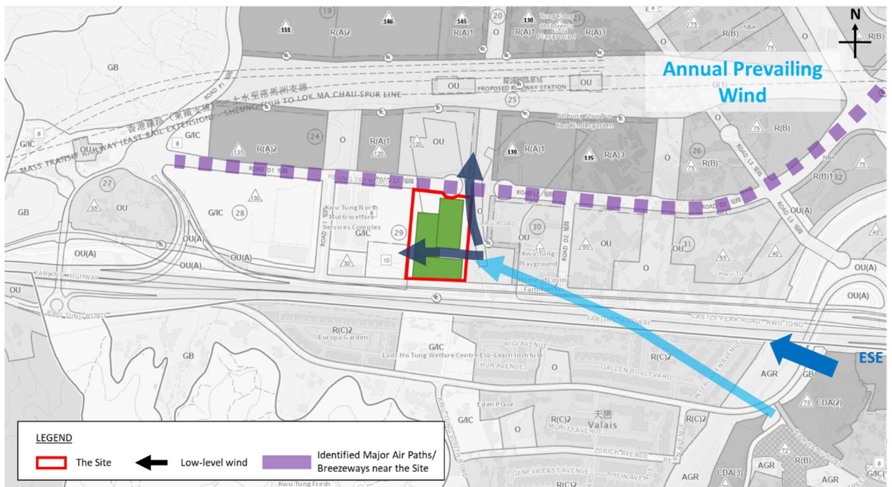
Figure 12 Major Air Paths under Proposed Scheme (ESE Wind)
