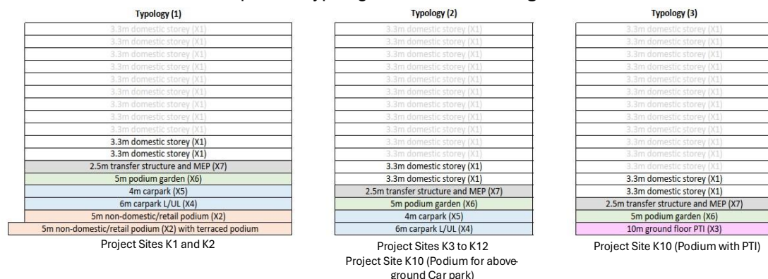
Figure 7.2 Indicative Sections of Different Types of Podiums within the Application Sites under the Proposed Scenario
