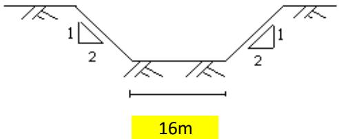
Area of flow  $A = 35.280 \text{ m}^2$  (Based on as-built drawing)
