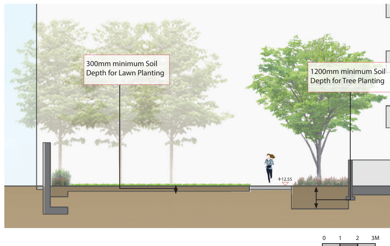
FIGURE TITLE S16 Planning Application for Proposed Residential Development cum RCHE and Shop and Services at various lots in D.D. 92 and 94 and Adjoining Government Land, Hang Tau Tai Po, Kwu Tung South Typical Section showing Soil Depth
