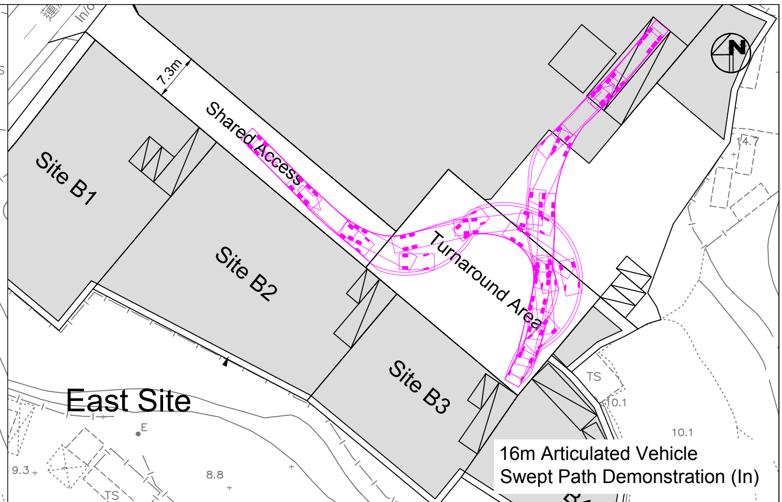
16m Articulated Vehicle Swept Path Demonstration (In)
