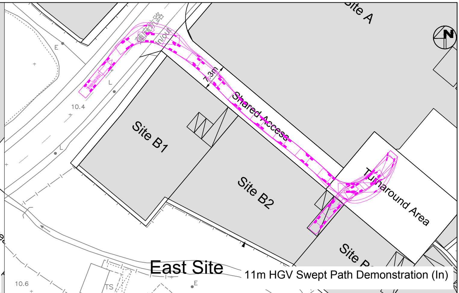
East Site 11m HGV Swept Path Demonstration (In-Step 1)
