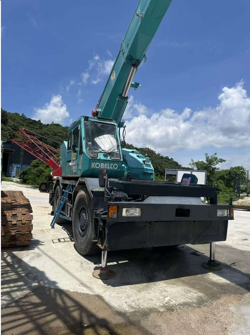
Figure 1: Wheeled hydraulic telescopic boom crane for supervised training and practical assessment.
