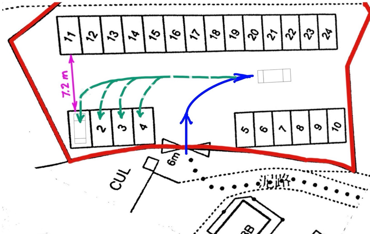
DIAGRAM 2.2.3.1 : RECOMMENDED MINIMUM STANDARDS OF TURNING CIRCLE FOR PRIVATE CARS
