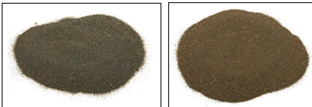
Photo 3.1 Photos of Columbite (Left) and Wolframite (Right) – Examples of Ore Minerals to be Stored in Premises
