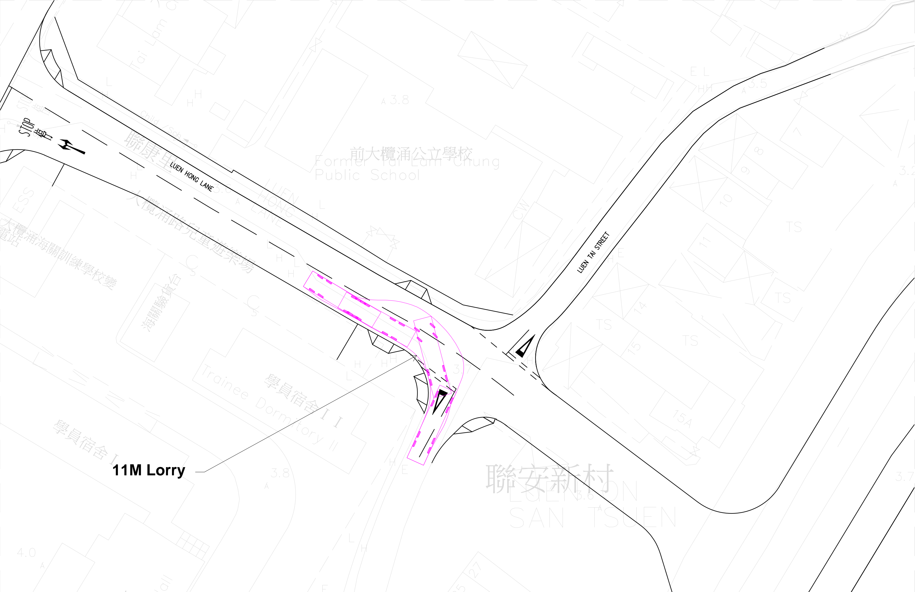
ANNEX C - SWEPT PATH DIAGRAM AT LUEN HONG LANE / LUEN TAI STREET JUNCTION 1:300 (A3) Annex C - SK9
