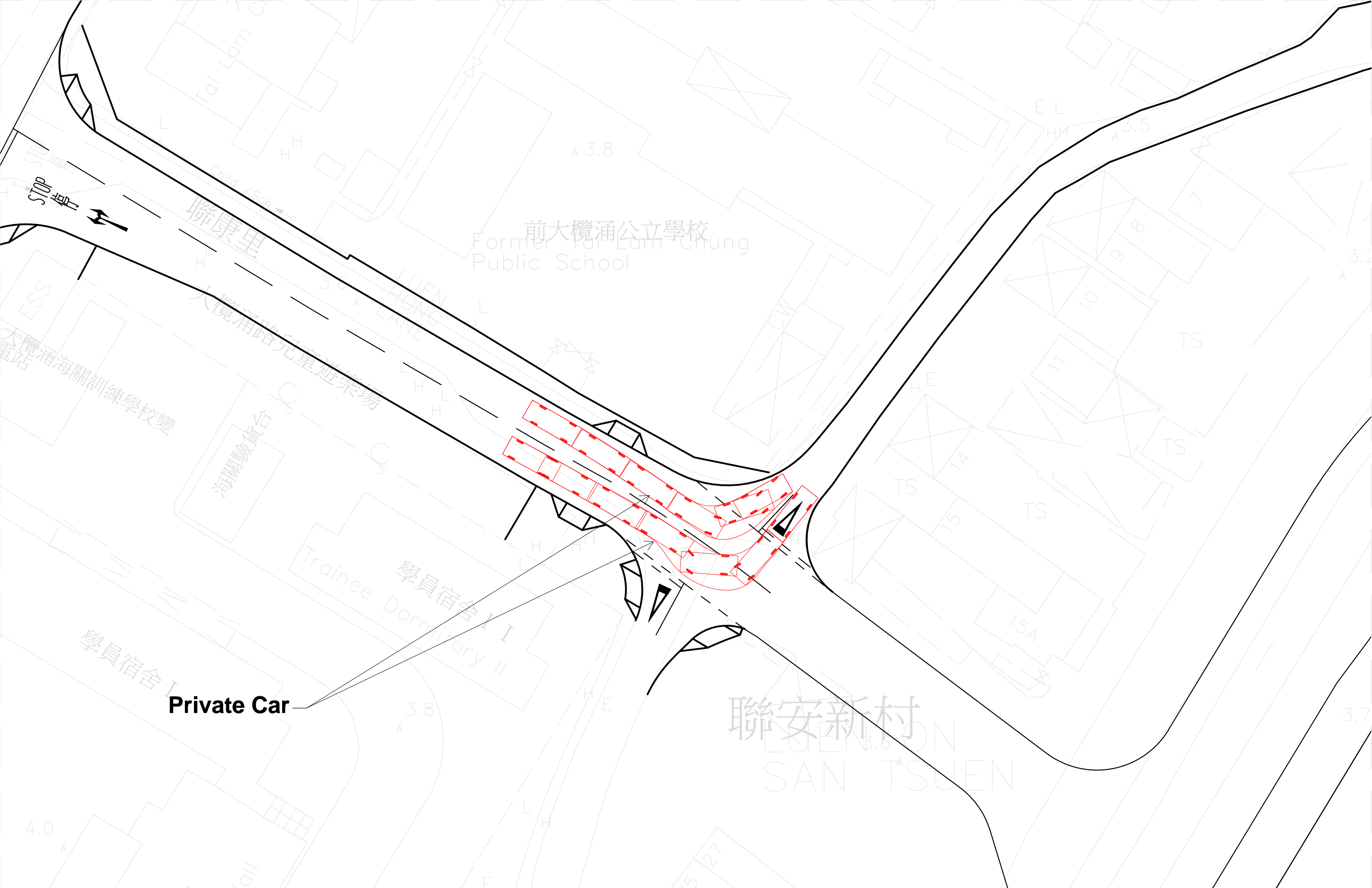
ANNEX C - SWEPT PATH DIAGRAM AT LUEN HONG LANE / LUEN TAI STREET JUNCTION 1:300 (A3) Annex C - SK8
