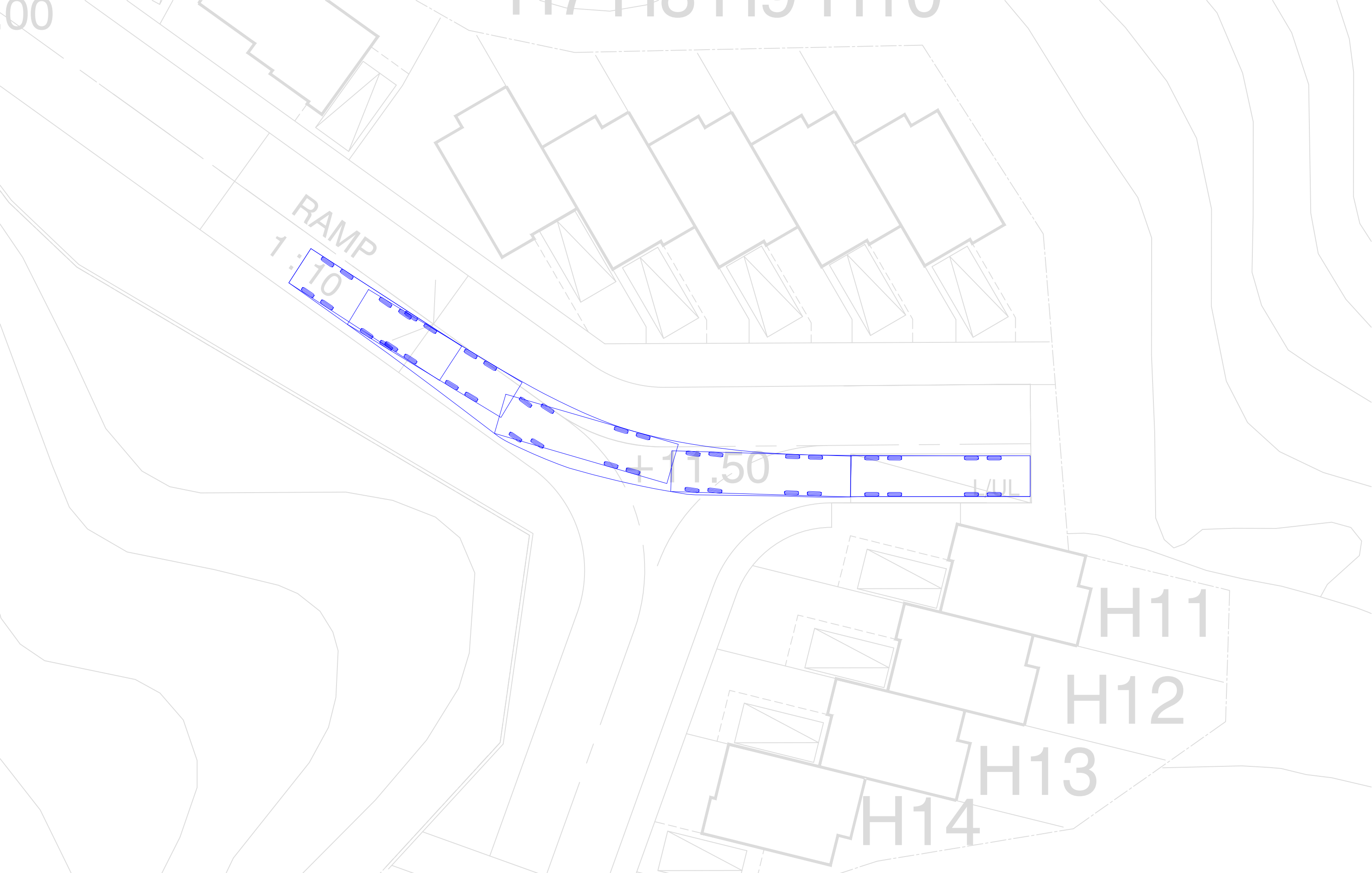
ANNEX C - SWEPT PATH DIAGRAM AT L/UL FOR 11m HGV (EGRESS) 1:300 (A3) Annex C - SK19
