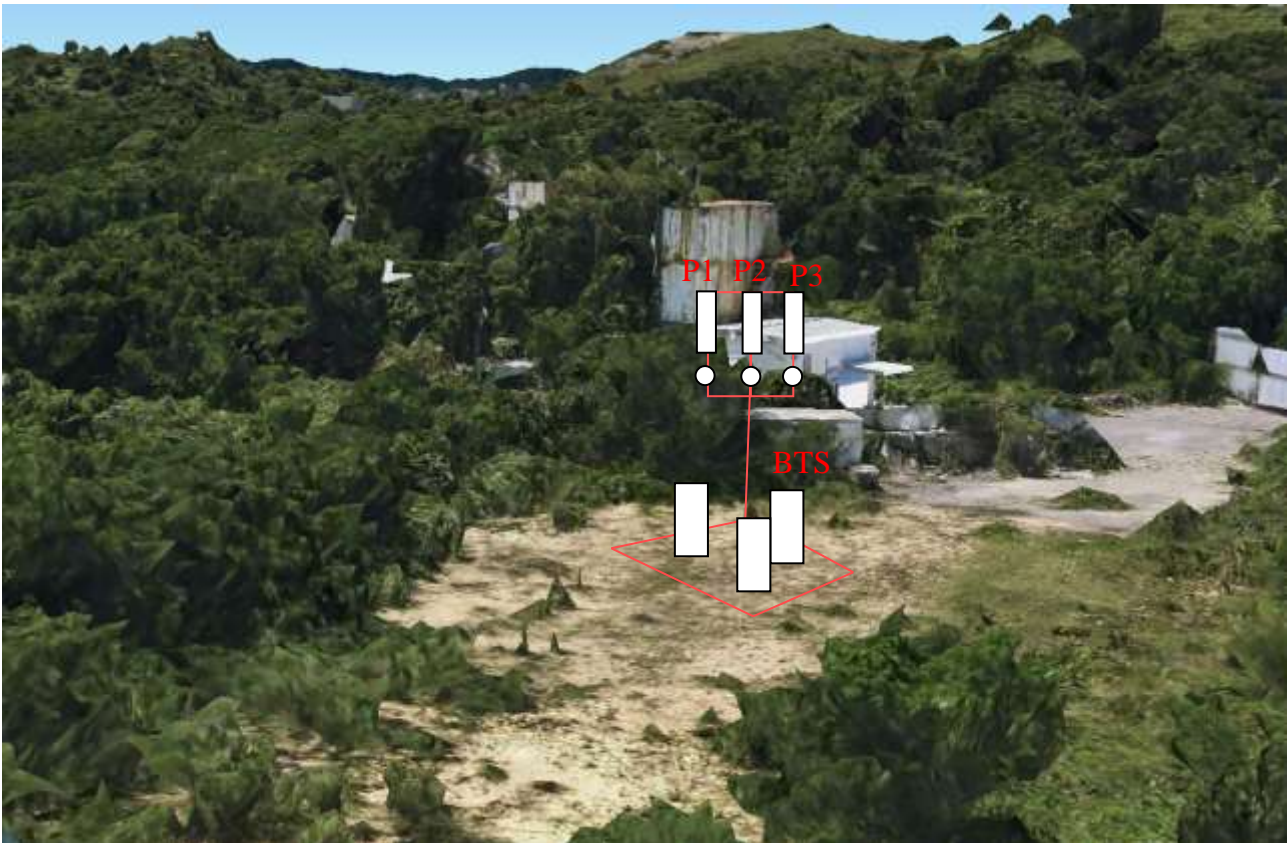
Photo 2: Proposed concrete plinth for BTS equipment and antenna posts P1 to P3 location
