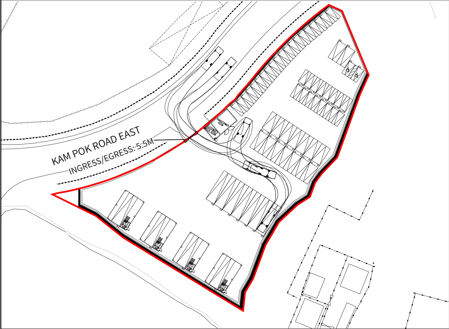
COACH ENTERING/EXITING SITE FROM THE WEST
