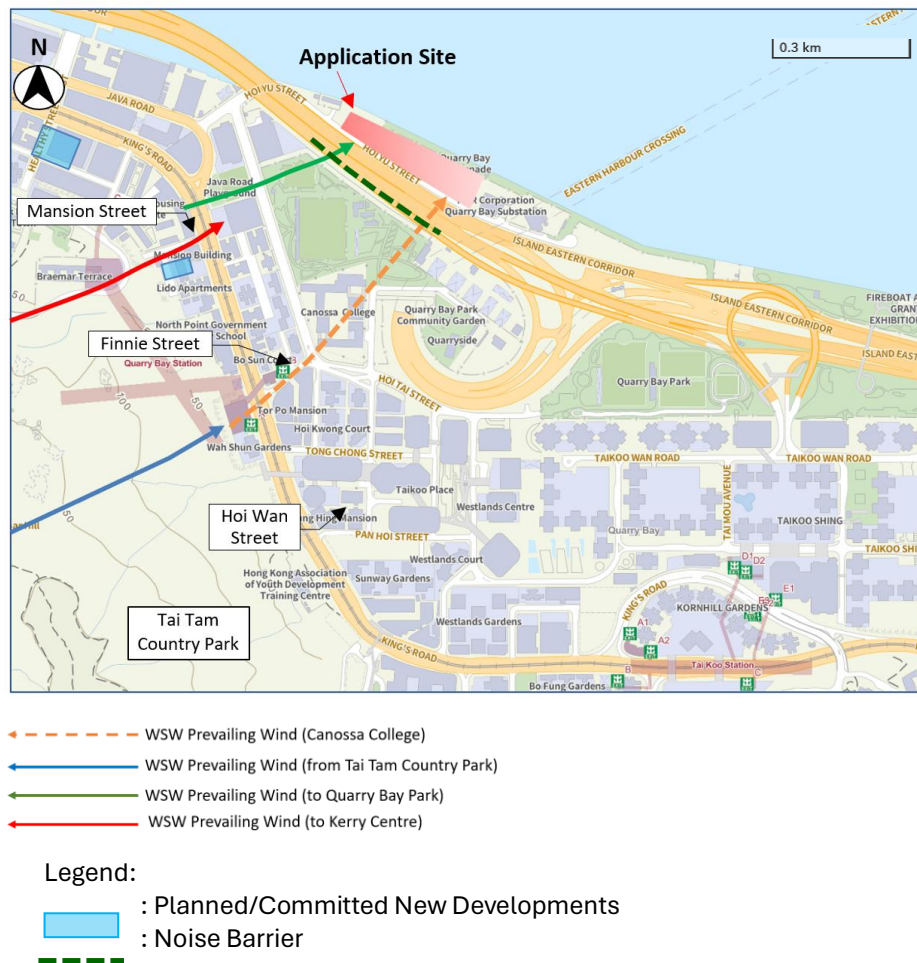
Figure 2-15 Wind Corridors Under Wind Direction WSW
