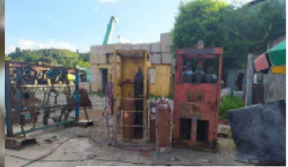
acetylene cylinders found (improper storage)
