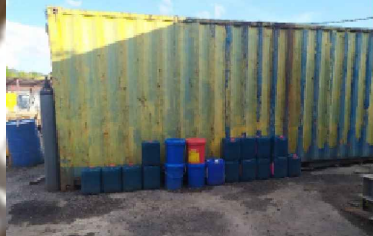
Waste oil container found (improper storage)
