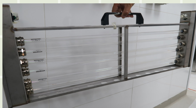
Cassette panel mounted with UV-C lamps
