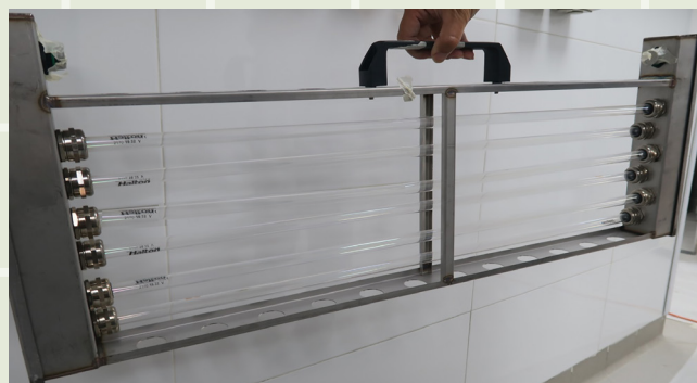
Cassette panel mounted with UV-C lamps
