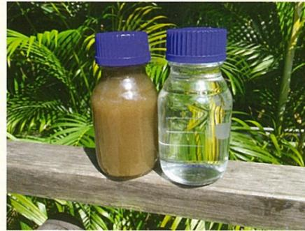
Raw wastewater (left) and treated water (right)
