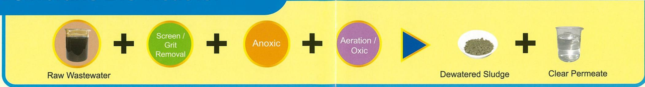
MBR is a new wastewater treatment technology, which combines biological treatment with membrane separation. In conventional activated sludge processes, the separation of the treated water from the sludge is mainly achieved by sedimentation in the secondary clarification tank. This requires a considerable amount of space and capital cost, and the separation efficiency is low.
