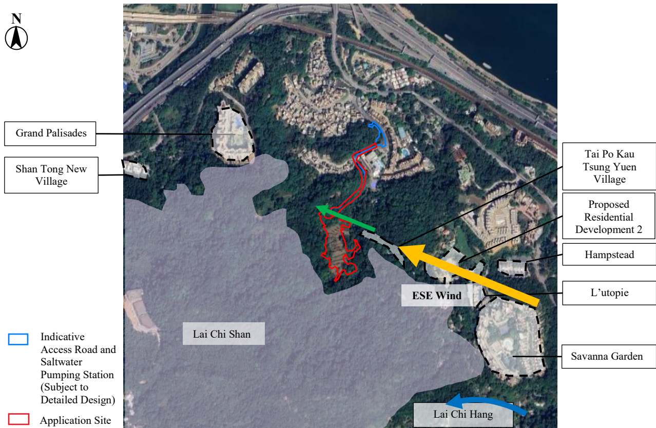
Figure 12 Wind Environment under ESE wind.
