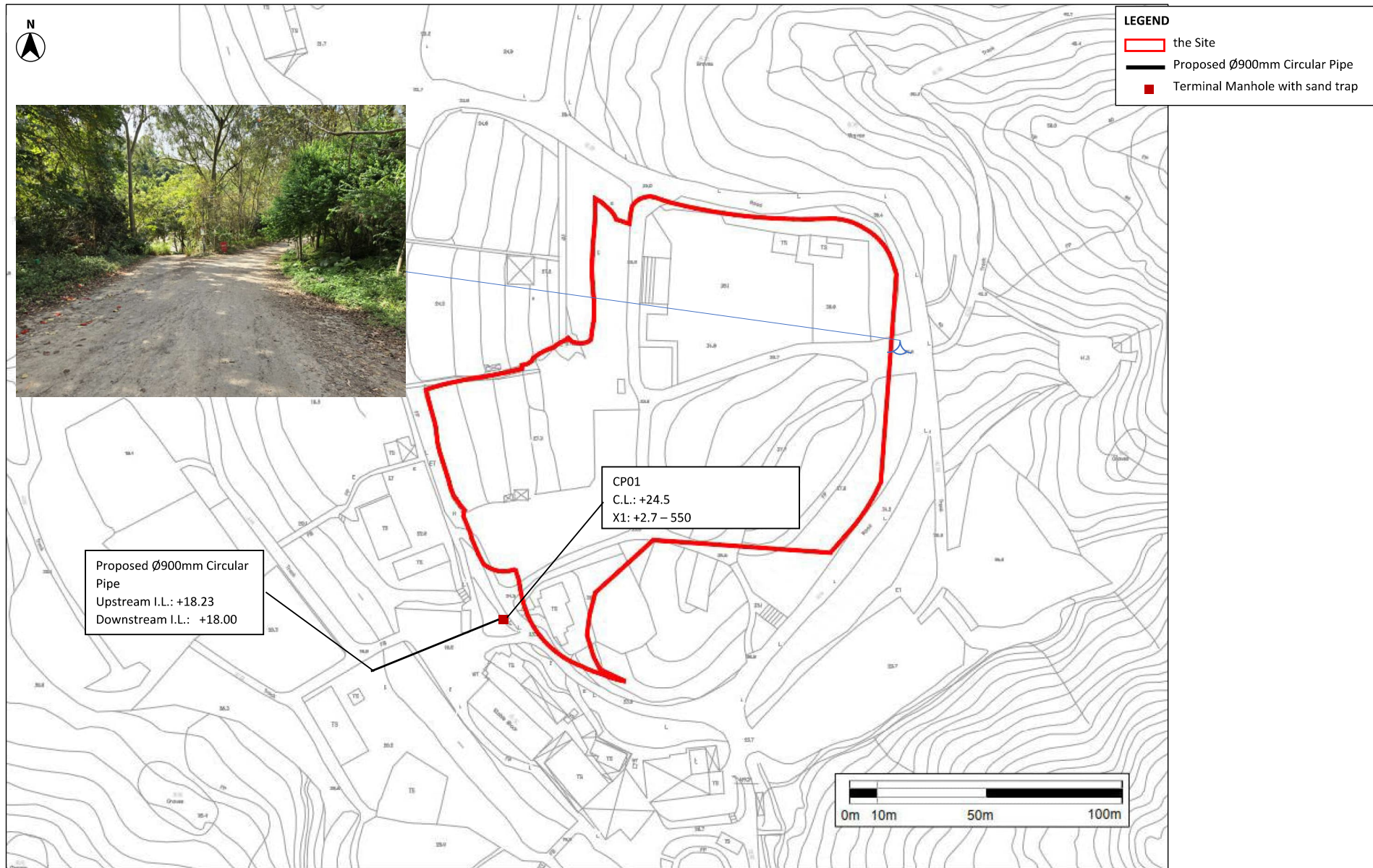
Figure 3-2 Indicative Location of Proposed Terminal Manhole and Stormwater Pipe
