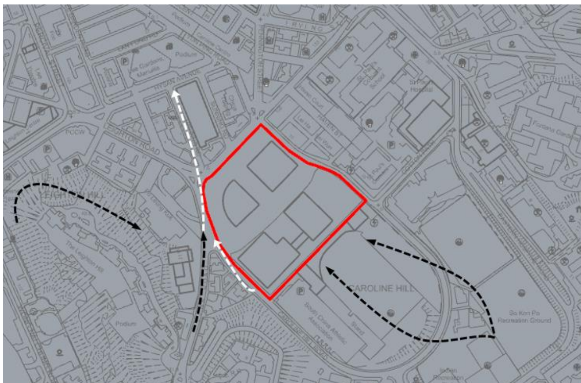
Figure 68 Major Air Paths under SW Wind for Proposed Scheme
