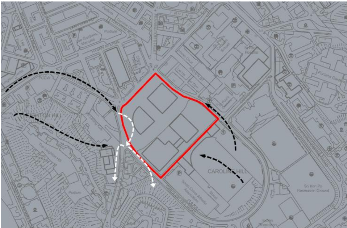
Figure 62 Major Air Paths under S Wind for Proposed Scheme
