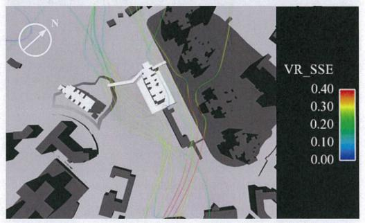
Figure 48 Streamline Plot for the Enhanced PRH Scheme (SSE Wind Condition)
