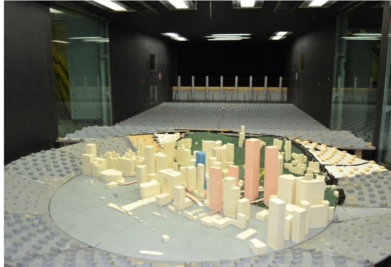
Figure 6 Wind tunnel model and setup, viewed from Northwest
