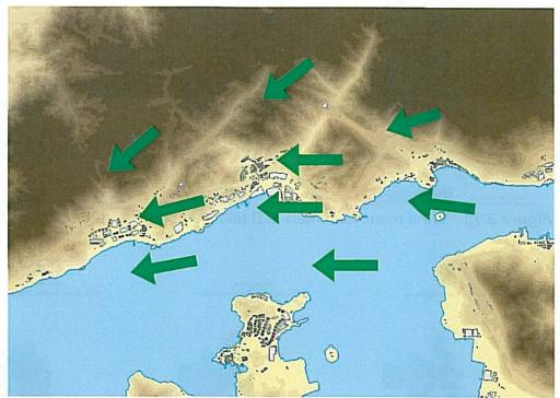
Figure 3.16 Prevailing wind directions at 60m (annual) based on MM5-CALMET model simulation.
