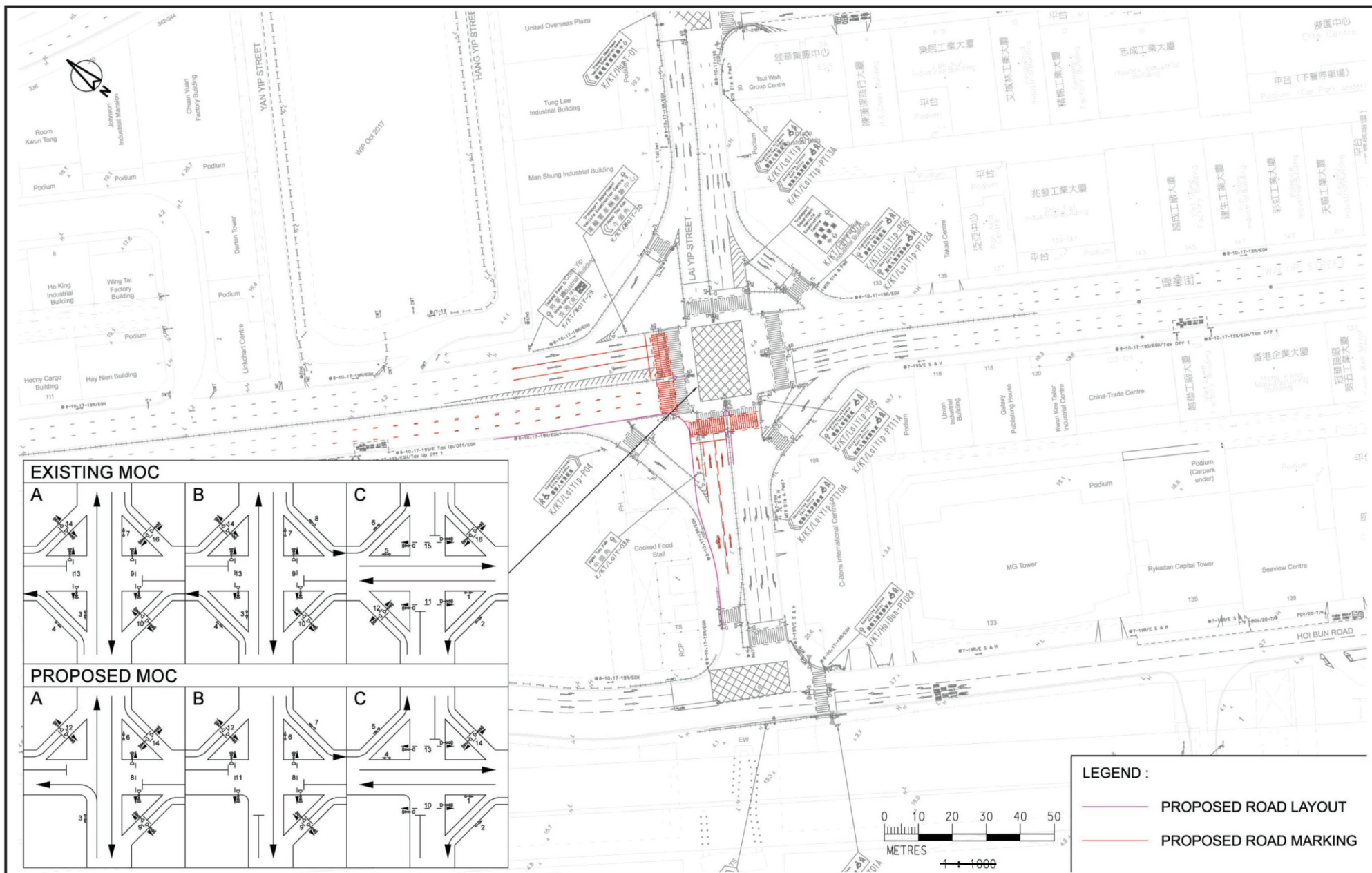
FIGURE 2.1.2 JUNCTION DESIGN FOR WAI YIP STREET / LAI YIP STREET JUNCTION (TO BE IMPLEMENTED BY OTHER PROJECT)
