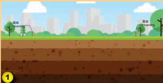
建造工程開始前，先整理工地現場及以圍板圍封工地 Tidy up and fence off the site by hoarding before commencement of construction
