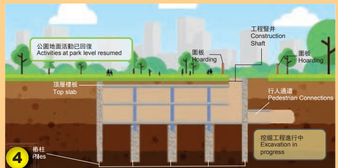
在重建和優化公園的同時，於地下繼續挖掘工作，並在合適的地方以無坑挖掘的方式建造行人通道 Continue the underground excavation works at the same time of reinstatement and facelift works. Conduct trenchless excavation for construction of pedestrian connections where suitable
