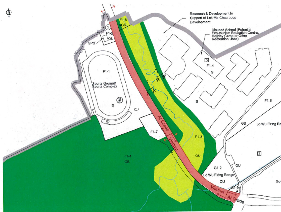
Figure 4 After stream diversion, the western riparian zone of Ma Tso Lung Stream would still be too narrow with only 15m (A to A'). Road R1 (red colour) is located right next to the stream (blue colour), thus encroaching part of its riparian zone 6 .
