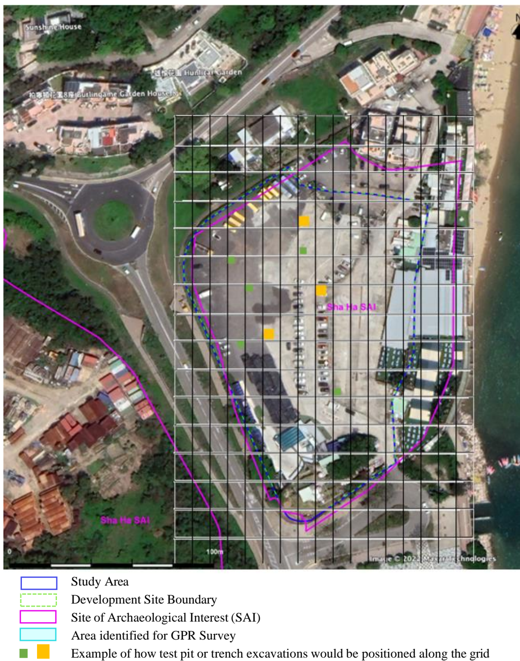
Figure 9 Aerial photograph showing Study Area and example of how test pit or trench excavations would be positioned along the grid within the Study Area. The area identified for GPR survey is also marked.
