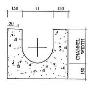
TYPICAL SECTION OF U-CHANNEL WITH COVER (N.T.S.)
