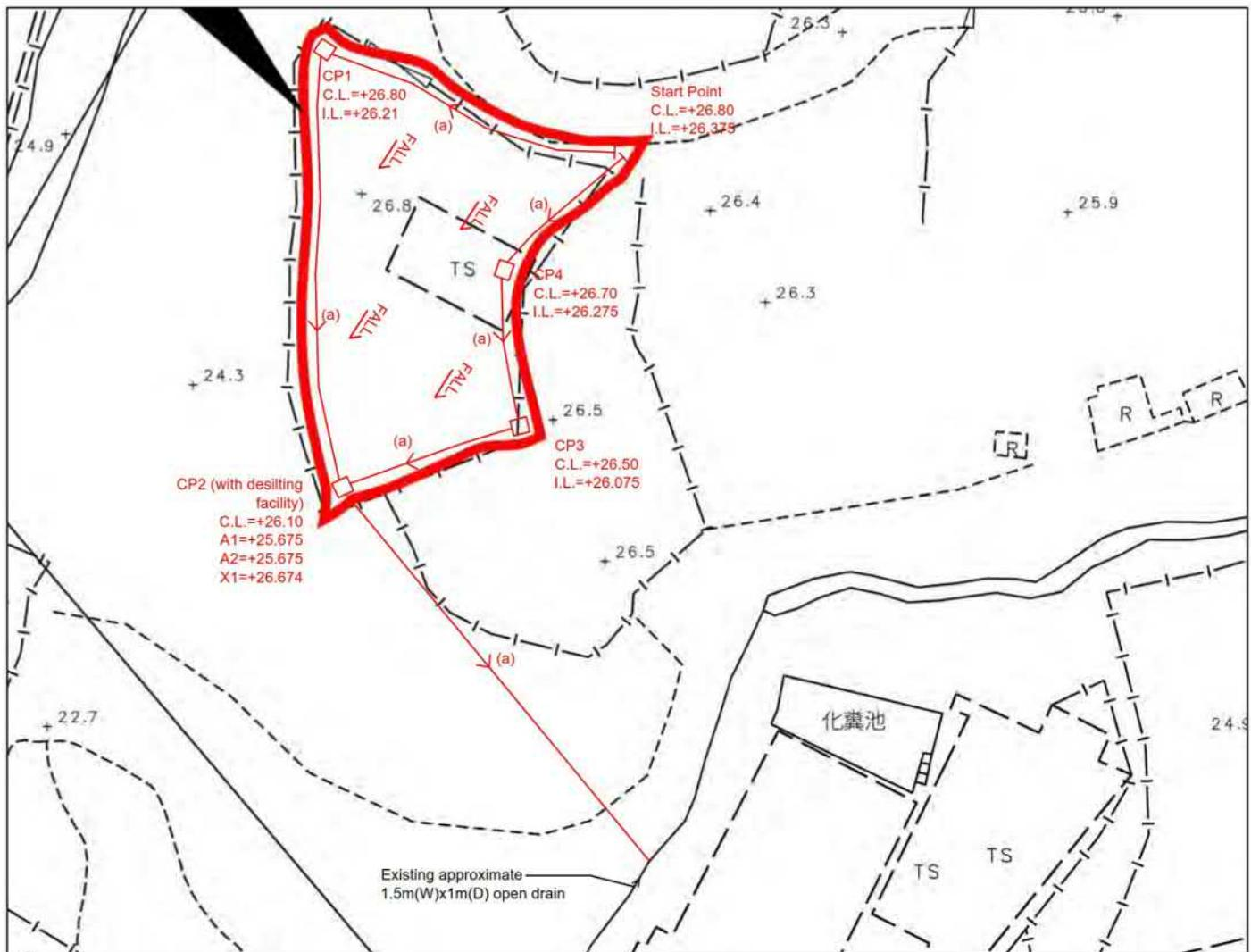
1. Catchpits (CP2) with desilting facility shall follow CEDD standard drawing No. C24061.
