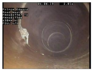
0001, 000327 Surface Damage Spalling Slight, from 08 to 09 o'clock Video Tape : Observation :
