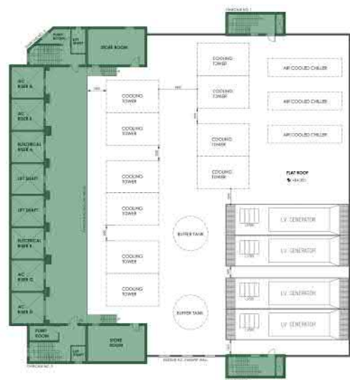
PROPOSED LAYOUT PLAN ROOF FLOOR PLAN TOTAL AREA AT R/F = 554.6377m 2
