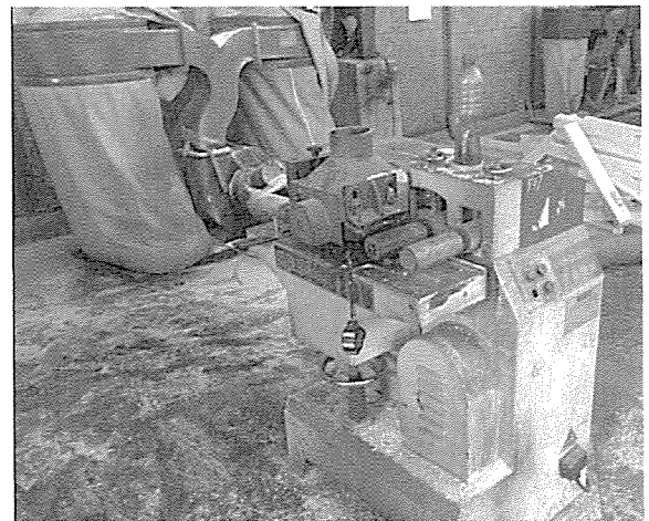
Photo 4: Single Face Planer (0.8m x 0.8m x 1.1m)
