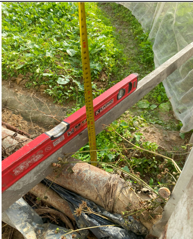
Photo View: A11 (Top of steel pipe is about 530mm high from the bottom of chaanel)
