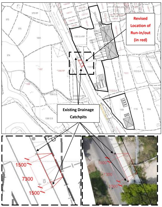
Designed design of the proposed run-in/out.
