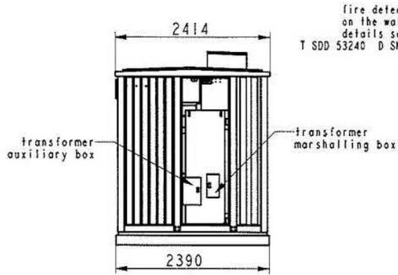
fire detection plate on the wall (300x300) details see drw. no : T SDD 53240 D SMS 1124 01-A
