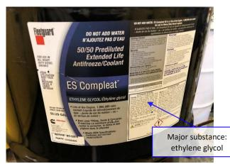
Photo 28: Label of the Anti-rust oil, antifreeze/coolant in Store Room 2
