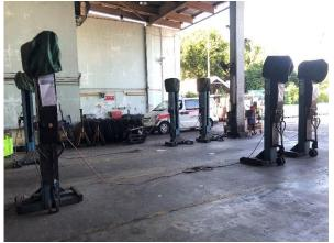
Photo 11: Lifting Equipment at Covered Parking Space
