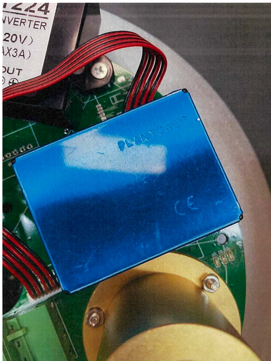
Photo E3. The Build-in Dust Sensors from Plantower (Beijing)
