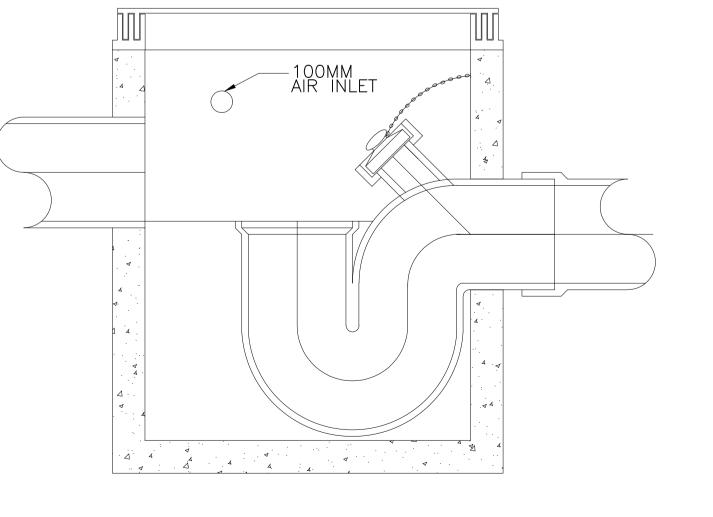
TERMINAL MANHOLE DETAIL (REFER TO DSD DWG <u>NO. DS(C)1058B)</u>
