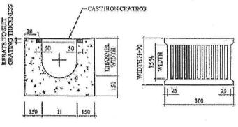
TYPICAL SECTION OF U-CHANNEL WITH COVER (N.T.S.)
