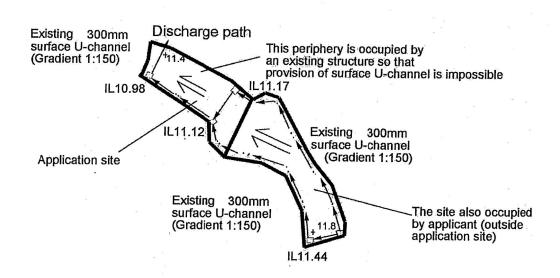
Project 項目名稱: Drawing Title 脚目: Remarks 備註: Proposed Temporary Shop (Grocery +<sub>11.4</sub> Level (in mPD) As-built Drainage Plan Store) for a Period of 3 Years at Lots Flow of surface runoff 1286 (Part), 1287 (Part), 1290 (Part), 1314 (Part), 1316 (Part) in D.D.119 & □ Proposed catchpit Adjoining Government Land, Pak Sha IL Invert level Drawing No. 關號: Tsuen, Yuen Long, N.T. Scale 比例: Figure 5 1:1000
