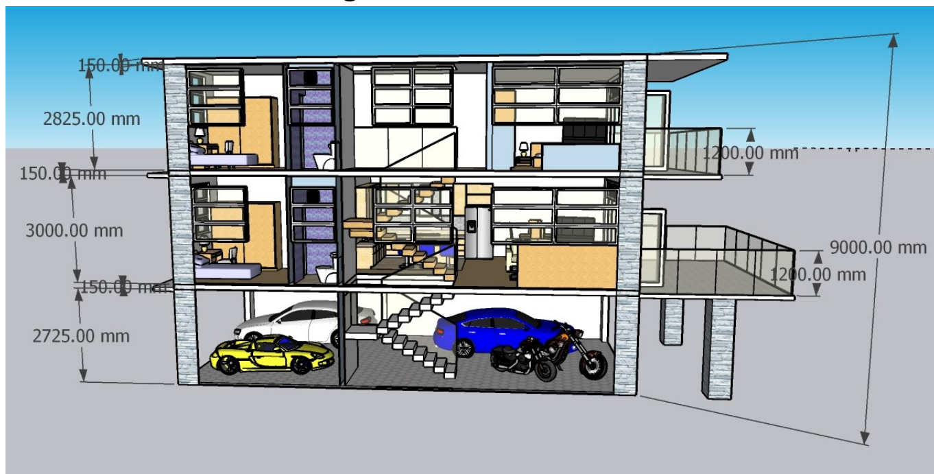
1 號屋橫切面尺寸圖，高度為 9 米 Cross Section Dimension Plan for House 1 and the max heigh is 9m
