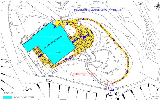
Figure 4.2 Pedestrian Management Plan (Extracted from Figure 3.1 of Traffic Management Plan)
