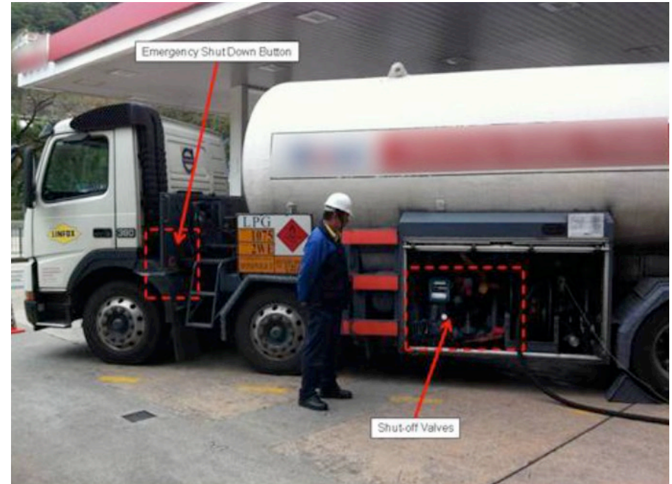
ESD button and shut-off valves on the LPG road tanker
